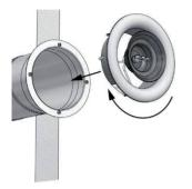
Press the body of the valve into the element and rotate it in a clockwise direction.
