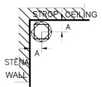
For piping with a diameter of 125 mm distance "A" from the wall and ceiling min. 150 mm.
