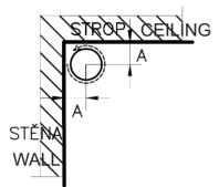
For piping with a diameter of 125 mm distance "A" from the wall and ceiling min. 110 mm.
