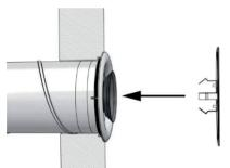
Lock the valve cone using a winged nut.
